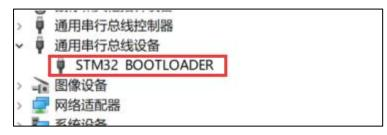
Before writing the firmware for the first time, you need to replace the STM32 BOOTLOADER driver to ensure that the OpenTX Companion software can recognize this hardware type and write the firmware correctly. The replacement method is as follows:
