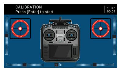
C. In the second step, place all the joysticks, knobs, and side sliders in the middle position. The system obtains the midpoint value, and then press the confirmation key to continue to the next step.
