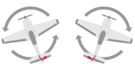
When the plane is rotated to left or right (Yaw), rudders should have the correcting actions as illustrated above.
