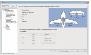
Options of wing types: Wing\_Rud\_Ele\_Ail----conventional model Wing\_Delta\_Ail/Wing\_Flying---- Delta/Flying wing
