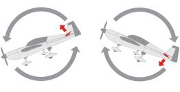
When the plane is rotated up or down (Pitch), elevators should have the correcting actions
